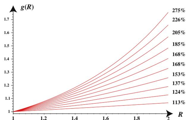
**Fig. 4** The cumulative growth function in the reference frame  $g = g(R)$ . We consider a growing elastic shell of initial radii  $R = 1$  and  $R = 2$ . Growth is linear in the current radius and chosen such that the inner shell experiences no growth  $g(R = 1) = 1$  and the total increment in volume is 1% at each step. The cumulative growth curves are shown for various values of volume increases. Note the marked super-exponential behaviour of  $g(R)$
