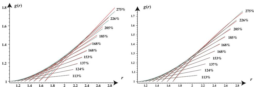
**Fig. 5** The cumulative growth as computed on Fig. 4 but now viewed in the current frame, that is,  $g = g(R(r))$ . Since the current configurations expands with growth the cumulative function  $g(r)$  can be fitted either with a linear (left) or quadratic fit (right)
