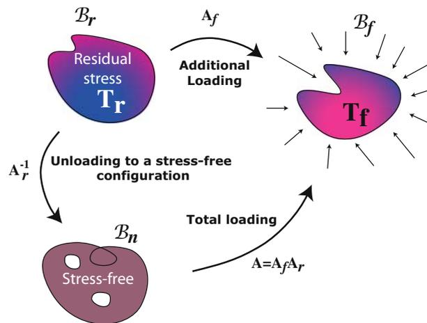
**Fig. 6** Computation of deformation for a pre-stressed body. First a stress-free configuration must be obtained from which the total loading is obtained as a composition of the two deformation gradients
