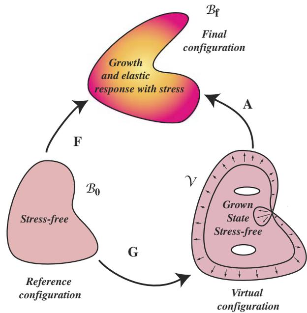
**Fig. 1** The decomposition of finite morphoelasticity. Starting from a reference configuration  $\mathcal{B}_0(\mathbf{X}, t)$ , the deformation gradient  $\mathbf{F}(\mathbf{X}, t)$  is the product of a growth tensor  $\mathbf{G}$  with an elastic deformation tensor  $\mathbf{A}(\mathbf{X}, t)$ . The intermediate configuration is referred to as a virtual configuration since compatibility and integrity cannot be ensured
