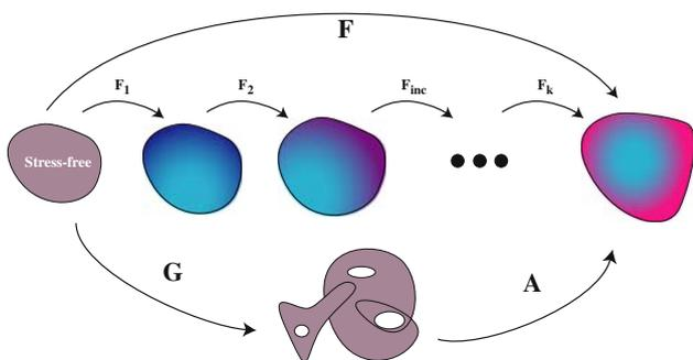
**Fig. 3** Computation of deformation for a pre-stressed body. First a stress-free configuration must be obtained from which the total loading is obtained as a composition of the two deformation gradients
