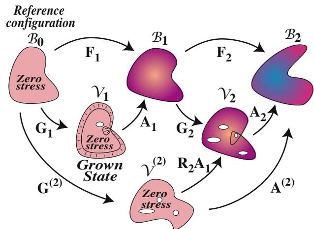
**Fig. 2** Cumulative growth with two steps, the superscript  $(k)$  denotes the total cumulative deformation after  $k$  incremental steps, whereas a subscript  $i$  denotes the incremental step taking place after the  $(i - 1)$ th step
