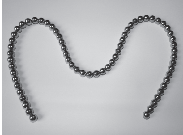
FIG. 1.1. Photograph of a chain of spherical magnets resting on a table-top. The diameter of the spheres in this image is 5 mm.
