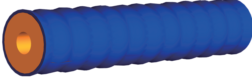
Figure 4: Schematic of the deformed model structure with transverse wrinkles.
